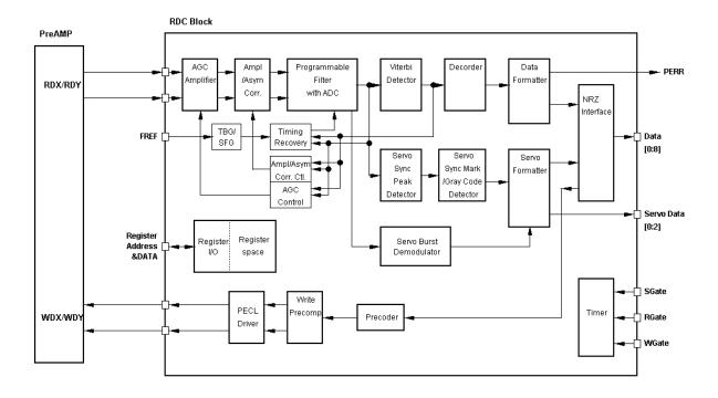
Figure 4.4 Read/write circuit block diagram
